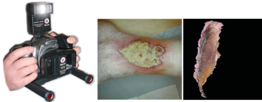
FIGURE 4.3: MAVIS-II THREE-DIMENSIONAL WOUND MEASUREMENT INSTRUMENT [48, 53]
